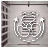
SmartWind ensures maximum evenness in cooking, thanks to the innovative thermodynamic fan design, together with intelligent management of the fan direction.
